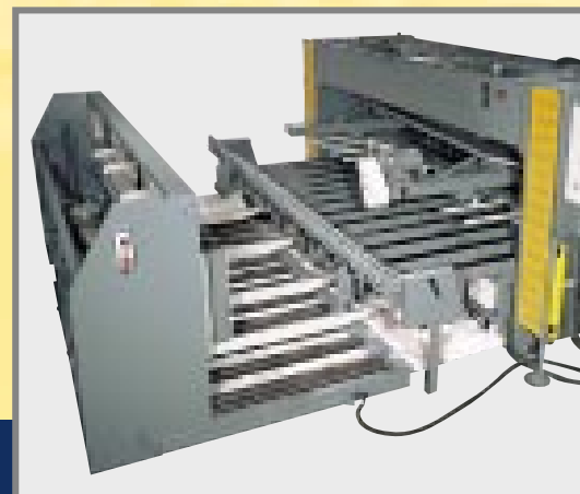
Pneumatic sheet hold-up system, scrap chute and scrap container, counter rolls, alignment cylinders and stacker with automatic adjustable arms.
