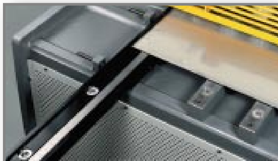
BALL TRANSFERS mounted in the iron table blocks, for easy feed-in of the sheets.
