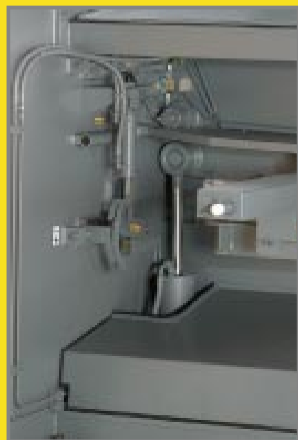
Picture including hydraulic blade gap setting (standard on TSX models with SC7 control unit)
